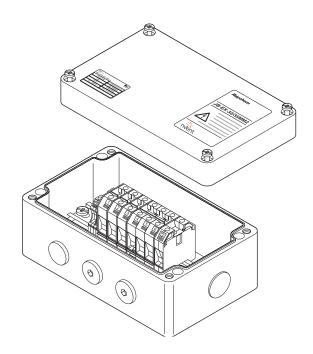
Industrial junction box for use in hazardous areas with MI heating cables when large terminal sizes are required. This box can be used to make connections between power cables, heating cables and cold lead cables. Depending on the configuration of the system, the box can accommodate multiple heating cables/cold leads and a power cable.
