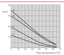
5BTV2-CR 3BTV2-CR 8BTV-2-CR 10BTV2-CR 3BTV2-CT **8BTV-2-CT** 5BTV2-CT **10BTV2-CT** Nominal power output (W/m at 10°C) 16 25 29 PRODUCT DIMENSIONS (NOMINAL) AND WEIGHT Thickness (mm) 5.5 5.5 5.5 5.5 Width (mm) 10.5 10.5 15.4 15.4 110 110 153 153 Weight (g/m)
