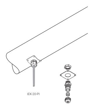
Insulation entry kits are designed to protect cables when passing through the thermal insulation cladding.
