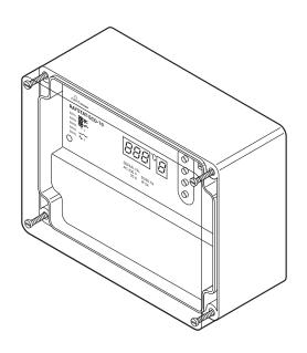
The nVent RAYCHEM RAYSTAT-ECO-10 temperature controller is designed to control heating cables used for frost protection applications. It continuously adjusts the heat-tracing output based on the ambient temperature. Using a proprietary algorithm, the RAYSTAT-ECO-10 controller measures ambient temperature and determines the appropriate cycle time during which the heating cables will be energised.
