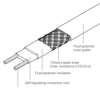
$1.4~\rm mm^2$  nickel plated copper conductors (10 and 15QTVR2-CT)  $2.3~\rm mm^2$  nickel plated copper conductors (20QTVR2-CT)
