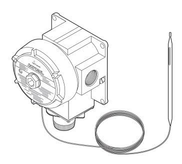
This EEx d approved surface sensing thermostat provides temperature control for all nVent RAYCHEM BTV, QTVR, KTV, VPL and XTV heating cables in hazardous areas. The switching temperature range is  $-4^{\circ}$ C to +163°C and is adjustable externally to the Ex enclosure by a dial mounted under a bolted-on cover and seal.
