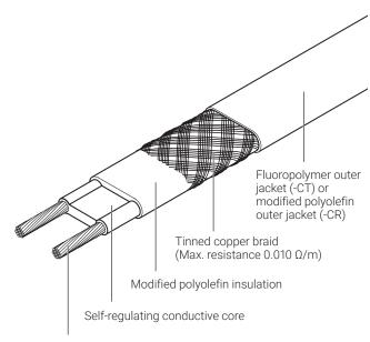
1.3 mm² nickel plated copper conductors
