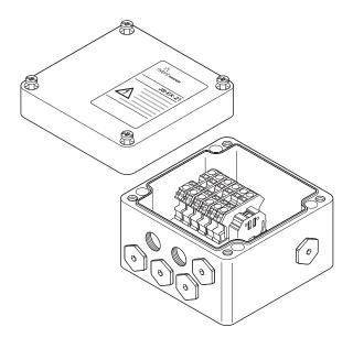
Industrial polyester junction box for use in hazardous areas. This box can be used to make connections between power cables, heating cables and cold lead cables using M20 connection kits. Depending on the configuration of the system, the box can accommodate six heating cables/cold leads and a power cable. M20 connection kits have to be ordered separately depending on the type of heating cable being used. Cable connection is accomplished via DIN rail mounted spring-type terminals.
