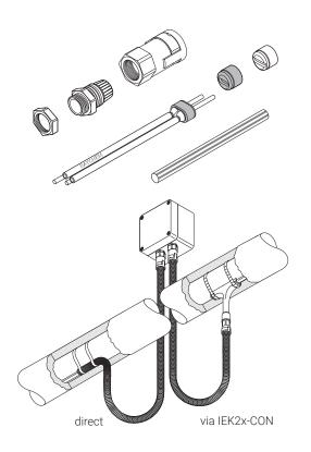
This connection kit is designed for terminating all nVent RAYCHEM BTV, QTVR, XTV, KTV and VPL parallel industrial heating cables to a junction box, whilst maintaining electrical insulation of the heating cable conductors and core as well as providing a reliable and sealed connection to a conduit system. It is approved for use in hazardous locations.
