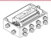
Remote Monitoring Modules (RMM2) provide temperature monitoring capability for the nVent RAYCHEM NGC-30 system.
