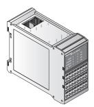
In addition to hardwiring an RTD directly into a Heat Trace Control module, RTDs can be wired to Input/output modules (NGC-40-IO) within the panel and assigned to heattracing circuits through software. This means that a nVent RAYCHEM NGC-40 system can be optimised for the specific application needs. Each IO module accepts up to four additional RTD inputs.
