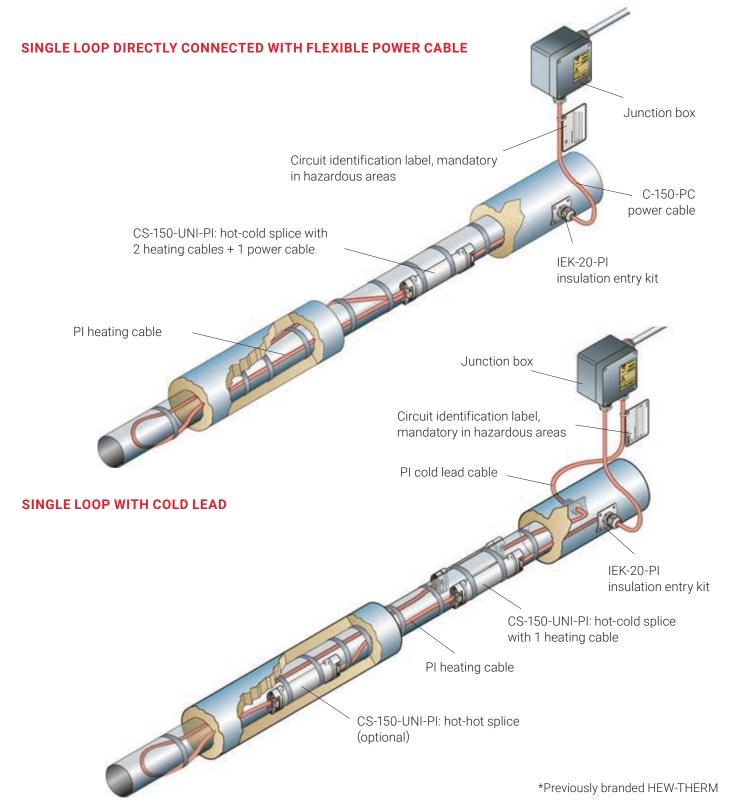
nVent offers Polymer Insulated heating cables in a very wide range of resistances as well as a complete range of components and accessories to build a complete heat-tracing system. All components are fully compatible across the three types and entire range of resistances.
