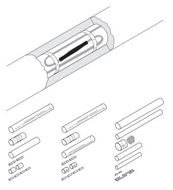
These splice kits are designed for the in-line joining of nVent RAYCHEM selfregulating heating cables.
