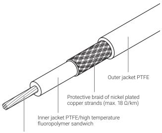
High temperature resistance heating conductor
