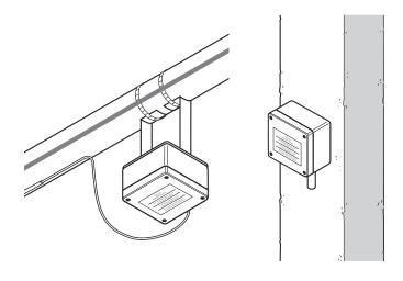
These electronic surface sensing and ambient thermostats provide accurate temperature control for heating cables.
