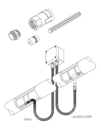
This connection kit is designed for terminating the full range of nVent RAYCHEM XPI polymer insulated series heating cables and cold leads in to a junction box, as well as providing a reliable and sealed connection to a conduit system.
