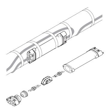
The nVent RAYCHEM S-150 is a cold applied low profile splice for in-line connection. This universal kit fits with all nVent RAYCHEM industrial heating cables, BTV, QTVR, XTV and KTV, meaning simplified product selection and reduced inventory to stock. It can be used in applications with temperatures ranging from -50°C to 215°C. It is approved for use in hazardous areas.
