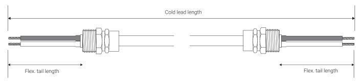
To facilitate occasional on-site termination and eventual repairs, nVent offers Pre-terminated MI double Cold Ends (PCE).
