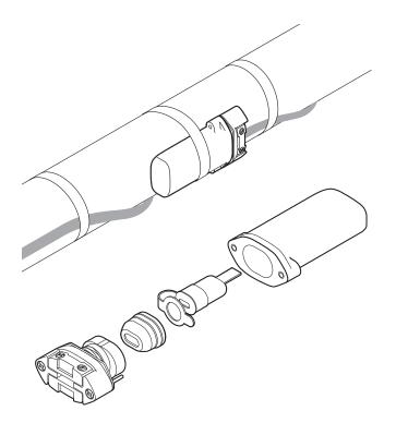
The nVent RAYCHEM E-150 is a cold applied low profile end seal. This universal end seal is designed to fit with all nVent RAYCHEM industrial self-regulating heating cables; BTV, QTVR, XTV and KTV meaning simplified product selection and reduced inventory to stock. It can be used in applications with temperatures ranging from  $-50^{\circ}$ C to 215°C. It is approved for use in hazardous areas.
