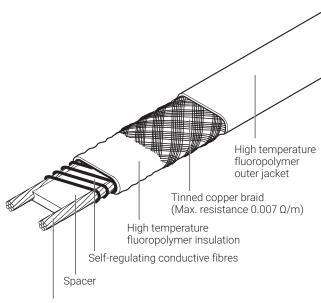
2.3 mm² nickel plated copper conductors
