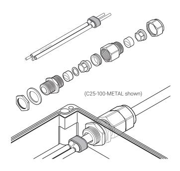
These connection kits are designed for terminating all nVent RAYCHEM BTV, QTVR, XTV, KTV and VPL industrial parallel heating cables to a junction box, whilst maintaining electrical insulation of the heating cable conductors and core.
