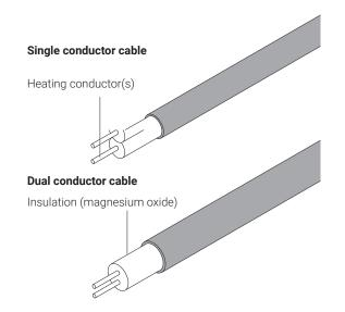
nVent RAYCHEM MI heating cables are available for a wide range of applications.
