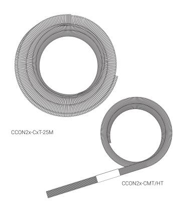
These conduits have been designed for use in combination with the conduit connection kits nVent RAYCHEM CCON2x-100-... They provide supplementary mechanical protection of the heating cable or cold lead between a junction box and the entry into the insulation. The conduit materials have been selected to meet the requirements for use in hazardous locations.
