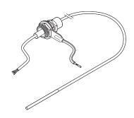
Certified EEx e II cable gland preinstalled on the sensor lead (M16, Brass, inclusive sealing washer, locknut and earth tag
