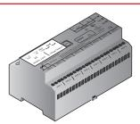
The nVent RAYCHEM NGC-40 works with the MONI-RMM2 module. Each RMM2 module installed in the field can accept up to 8 RTDs. 16 RMM2 Modules can be daisy chained together via RS-485 for a total of 128 temperature inputs. Since multiple RMM2s can be networked over a single cable to the nVent RAYCHEM NGC-40, the cost of RTD field wiring will be significantly reduced.
